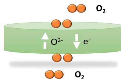
$T_{oper} = 500-800^\circ C$
